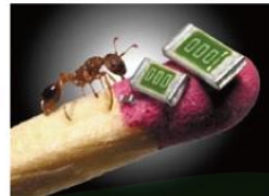
Figure 1. The size of an 0201 component as compared to an 0605 component, an 0603 component, an ant and a matchstick.
