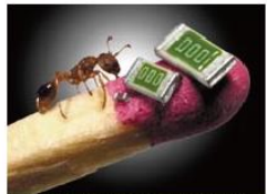
Figure 1. The size of an 0201 component as compared to an 0805 component, an 0603 component, an ant and a matchstick.
