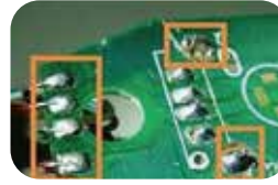
Cold Solder Joint
