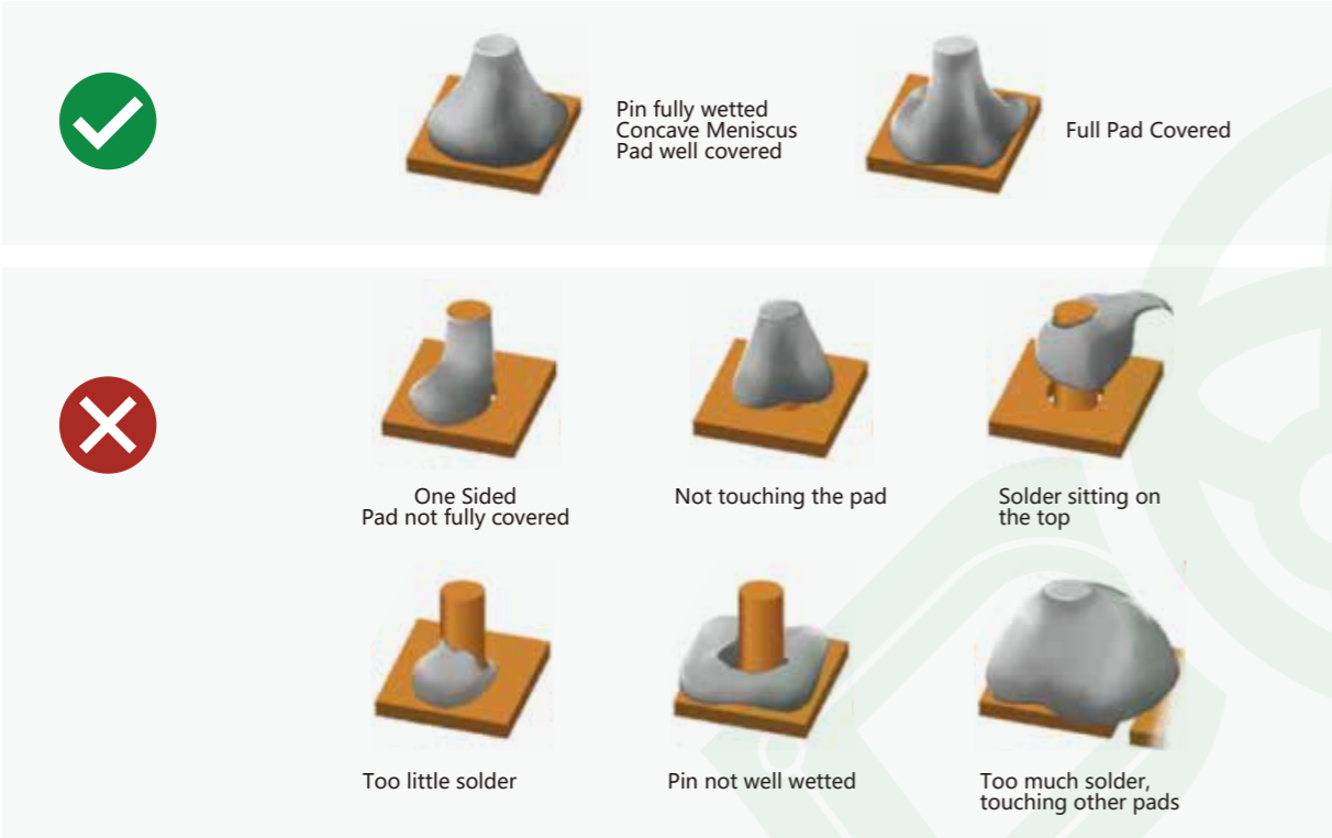
Soldering defects on a circuit board
